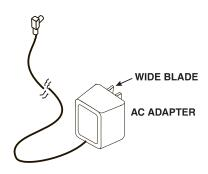
Do not alter the shape of the blades of the polarized plug.
